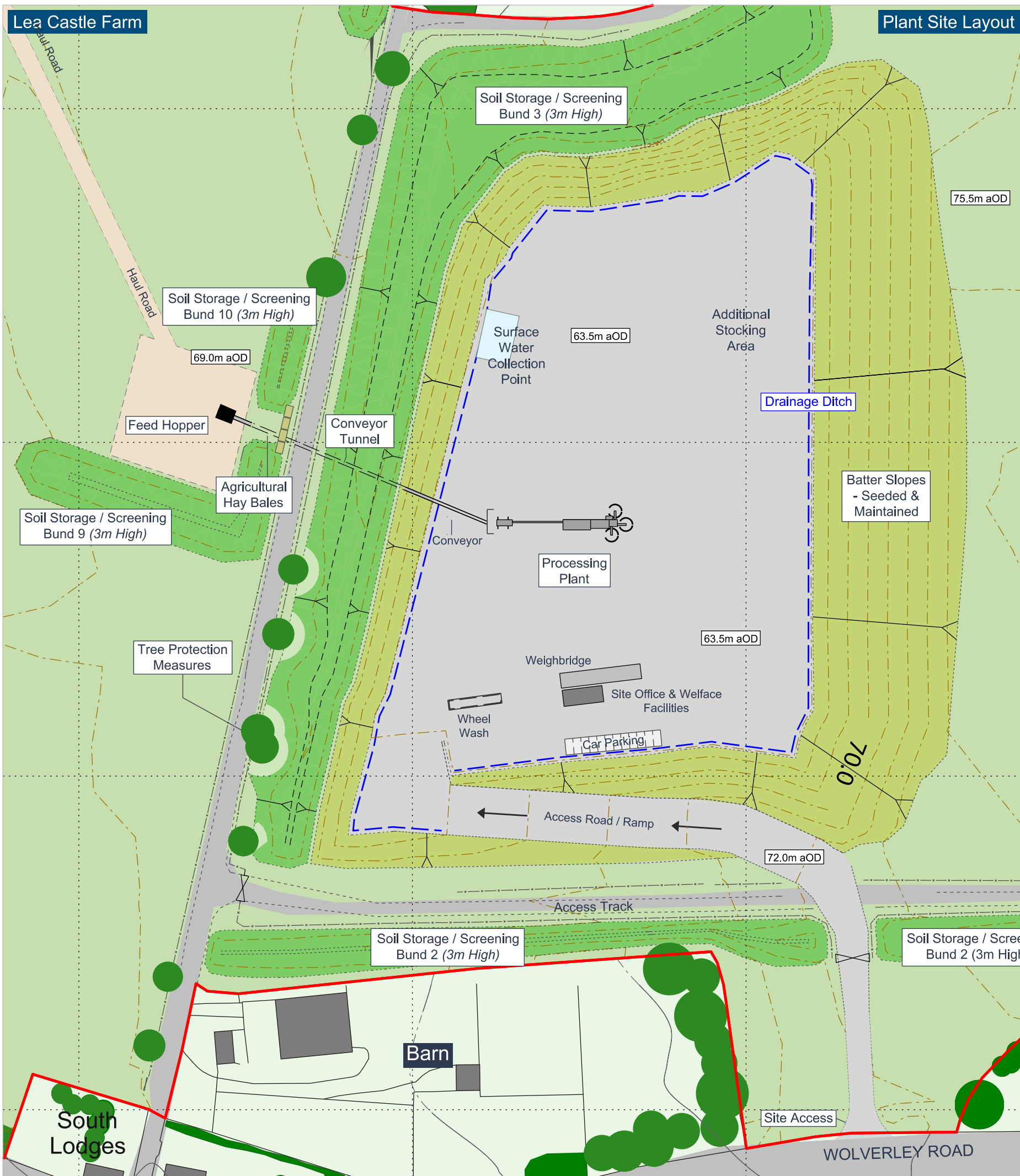
Plant Site - Footprint & Elevations (1:500 @ A3)
