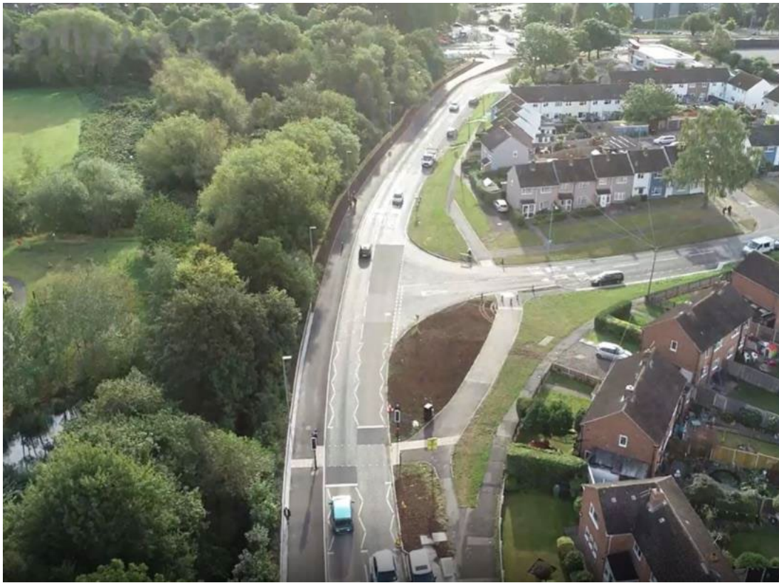
* An ariel photo of scheme 2b with cycle / pedestrian link and new Toucan Crossing up to A38.
