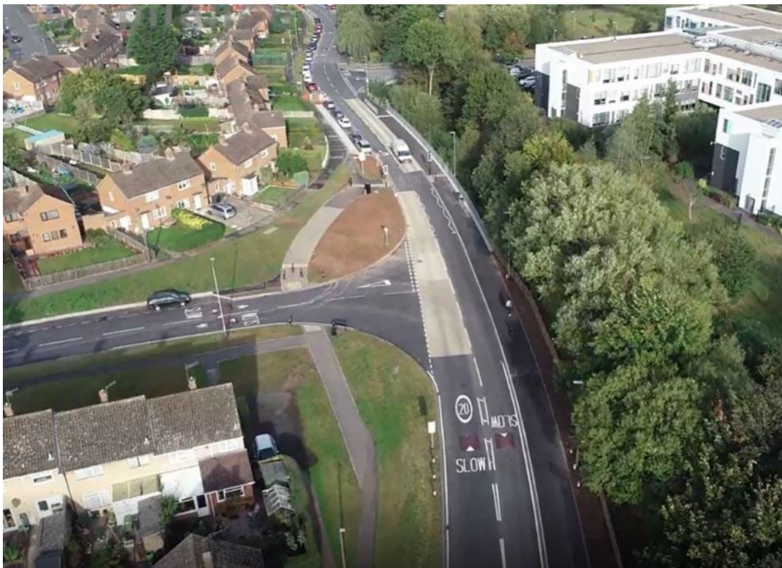
* An ariel photo of scheme 2b with cycle / pedestrian link and new Toucan Crossing connecting A38 to South Bromsgrove High School.
