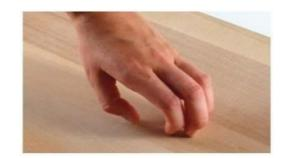
1, The free hand holds the material to be cut. The fingertips face the rear inside of the palm so cutting your fingers can be avoided.
