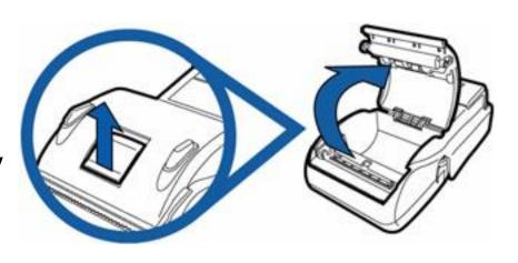
Place the new roll of paper as seen in the picture with the end of the paper going the correct way for the machine. This may change from machine to machine so look at how the paper comes out.
