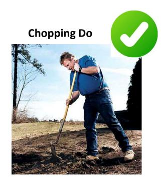
DO flip a long-handled, round-point shovel around so the head faces you to cut roots or clean up the sides of a hole. This orients the back of the shovel parallel to the sides of the hole, allowing you to chop downward with great force.
