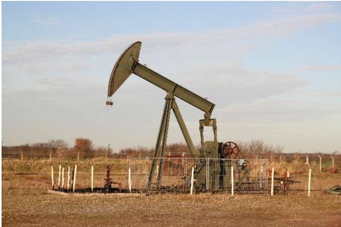
Figure 4: Beam Pump. (Photo copyright Richard Croft, Creative commons Attribution - ShareAlike 2.0 licence)
