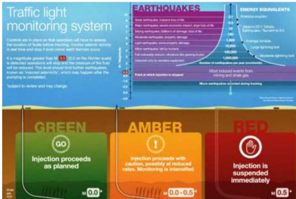
Figure 3: Traffic light monitoring system for seismic events related to fracking. 62
