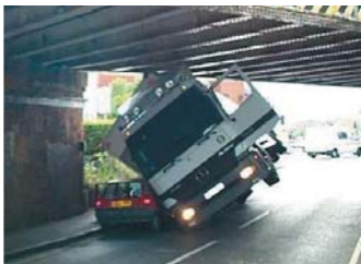
A crushed car as a result of a bridge strike
