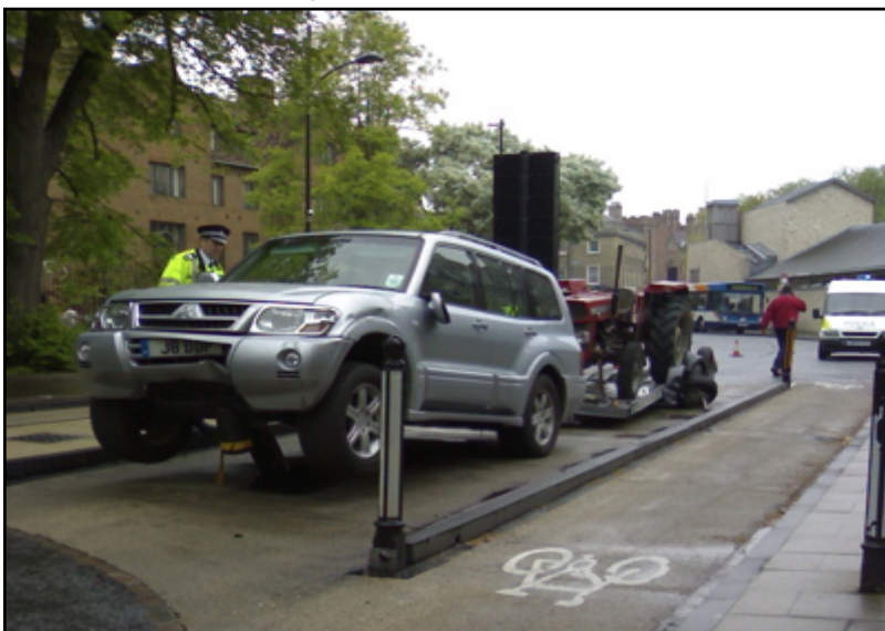
Figure 7.1 - Violation of a Rising Bollard
