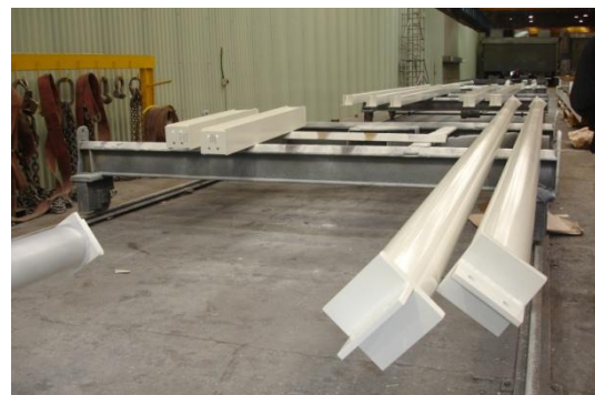
Finished painted steel columns
